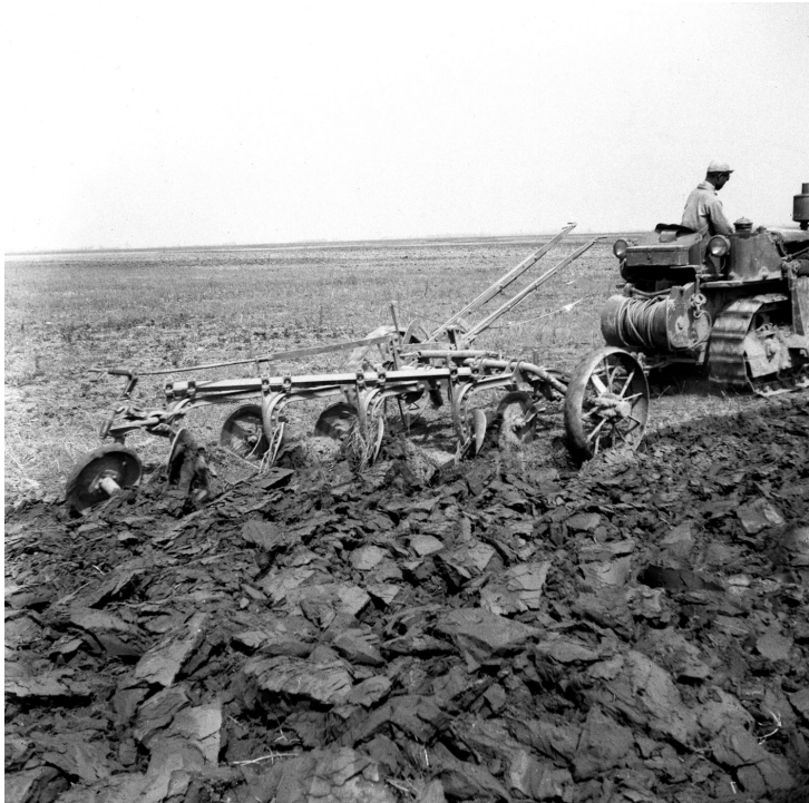
A 4-share plow being pulled by a sturdy little war surplus tractor. (UNRRA photograph.)
